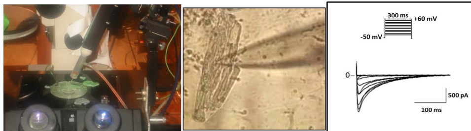
Patch-clamp technique used to record L-type \text{Ca}^{2+} current in Ventricular cardiomyocytes isolated from a mouse heart
